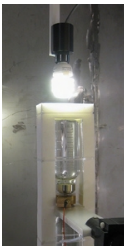
Figure 2: Liquid-filled phantom in the electrical field of the energy-saving lamp. The currents induced in the phantom are measured using the clip in the middle. There is a gap of 2 cm between the bulb and the phantom [2].
