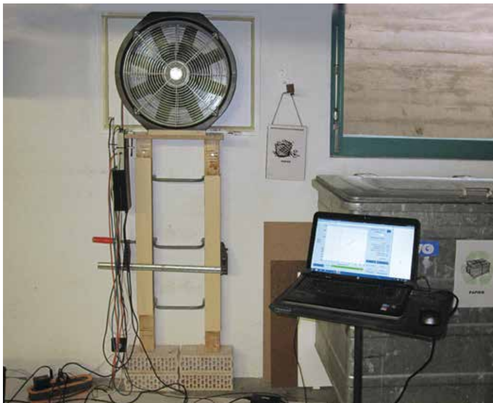
Figura 6.49: Test blower door.
