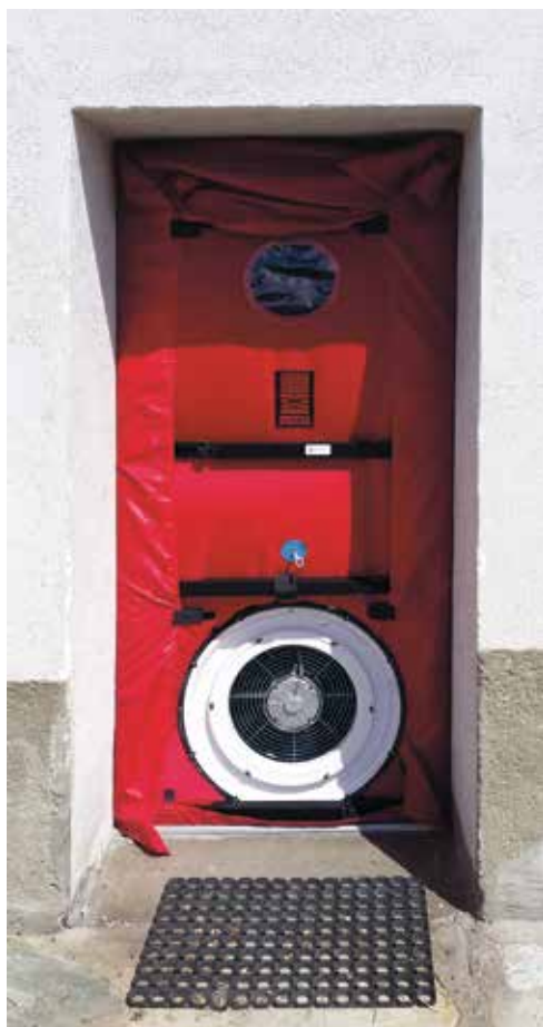
Figura 6.37: Test blower door.
