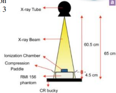
Equipment setup for (a) mean glandular dose measurement Malays J Med Sci. 2013 May; 20(3): 23–30.
