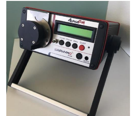
AlphaPM: Measuring Device for Equilibrium Factor
