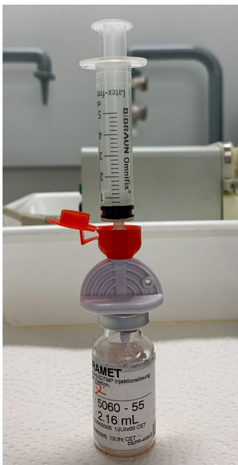
Figure 1. A vented Mini-Spike® Chemo with filter enabled safe injection of 4 M HNO 3 in a spent Quadramet vial without loss of radioactivity to the environment. Withdrawal of solubilised Eu from the vial was carried out using the same Mini-Spike®, minimising contamination risk through reduced amount of material.
