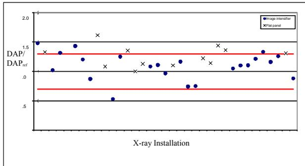
Fig. 1 Characterization of the DAP-meters of the x-ray installations to a reference chamber, red lines indicate  $\pm 30\%$  of the reference
