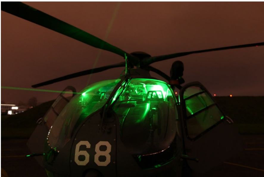
Figure 1: Dazzling effect with a laser pointer on the cockpit of a helicopter
