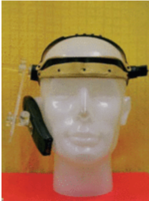
Figure 2: Head phantom for determining the SAR value. Photo source: [13] [13]
