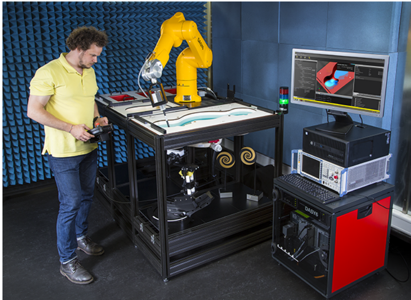
Figure 1: DASY6 dosimetric assessment system with the SAM and flat phantoms for SAR assessments according to [10], [11].
