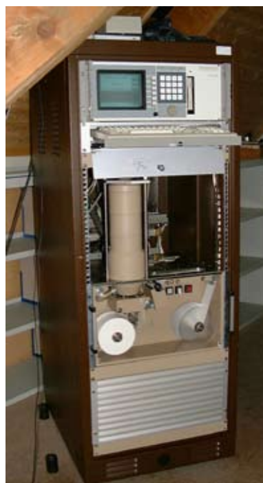
Photo 4: Station RADAIR de Sion (VS): Moniteur Alpha-Beta (FHT-59s)
