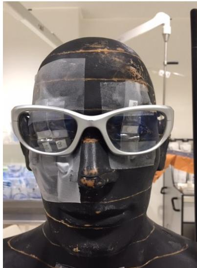
Figure 4. Representation of the scenario used for the measurement of the DRF when using goggles or RP face mask.
